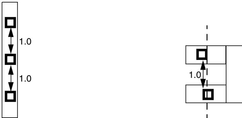
d) Okay. Cuts overlap, but share the same metal above or below; therefore `PARALLELOVERLAP` rule does not apply, and only 1.0 spacing is needed.
