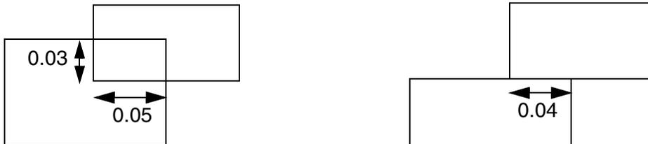
c) OK, the right direction width of 0.05 ( $\geq 0.05$ ) is met although the wrong way direction width fails
