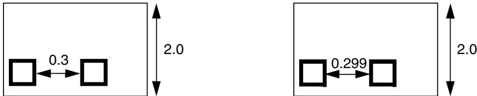
a) Violation. The wire width is  $> 1.0 \mu\text{m}$ , therefore 2 cuts are needed. However, the 2 cuts are  $\geq 0.3 \mu\text{m}$  apart, therefore they cannot be counted together.
