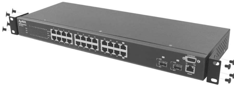
Figure 7 Attaching the Mounting Brackets
