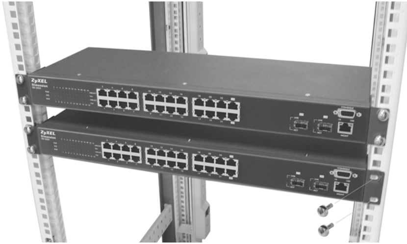
Figure 8 Mounting the Switch on a Rack
