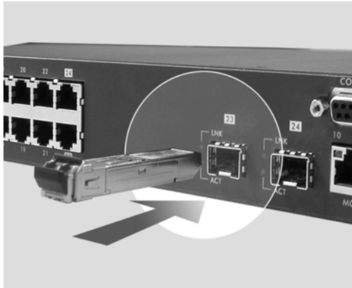
Figure 10 Transceiver Installation Example
