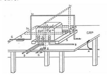
GRP: Ground plane C1: Power supply circuit
