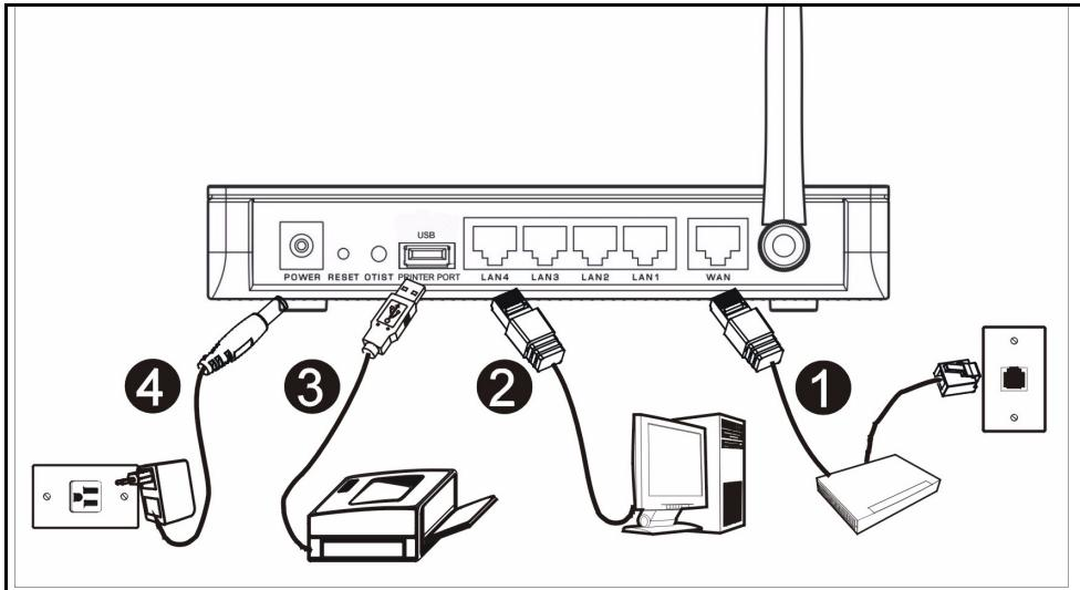
Do the following to make hardware connections for initial setup.
