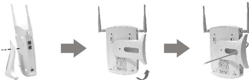
Figure 9 Support Holder Connections
