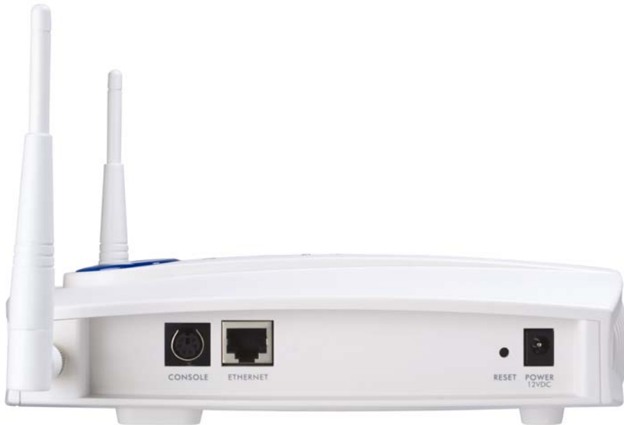
Figure 1 ZyAIR Side Panel and Connections
